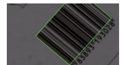
Reading strongly blurred bar codes.
